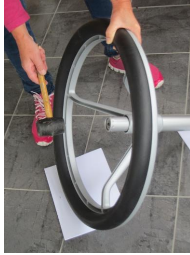
With a plastic hammer knock loose the pneumatic cylinder
